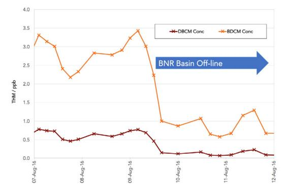
Figure 4: City of Paso Robles WWTP BNR Maintenance Effect on THMs
